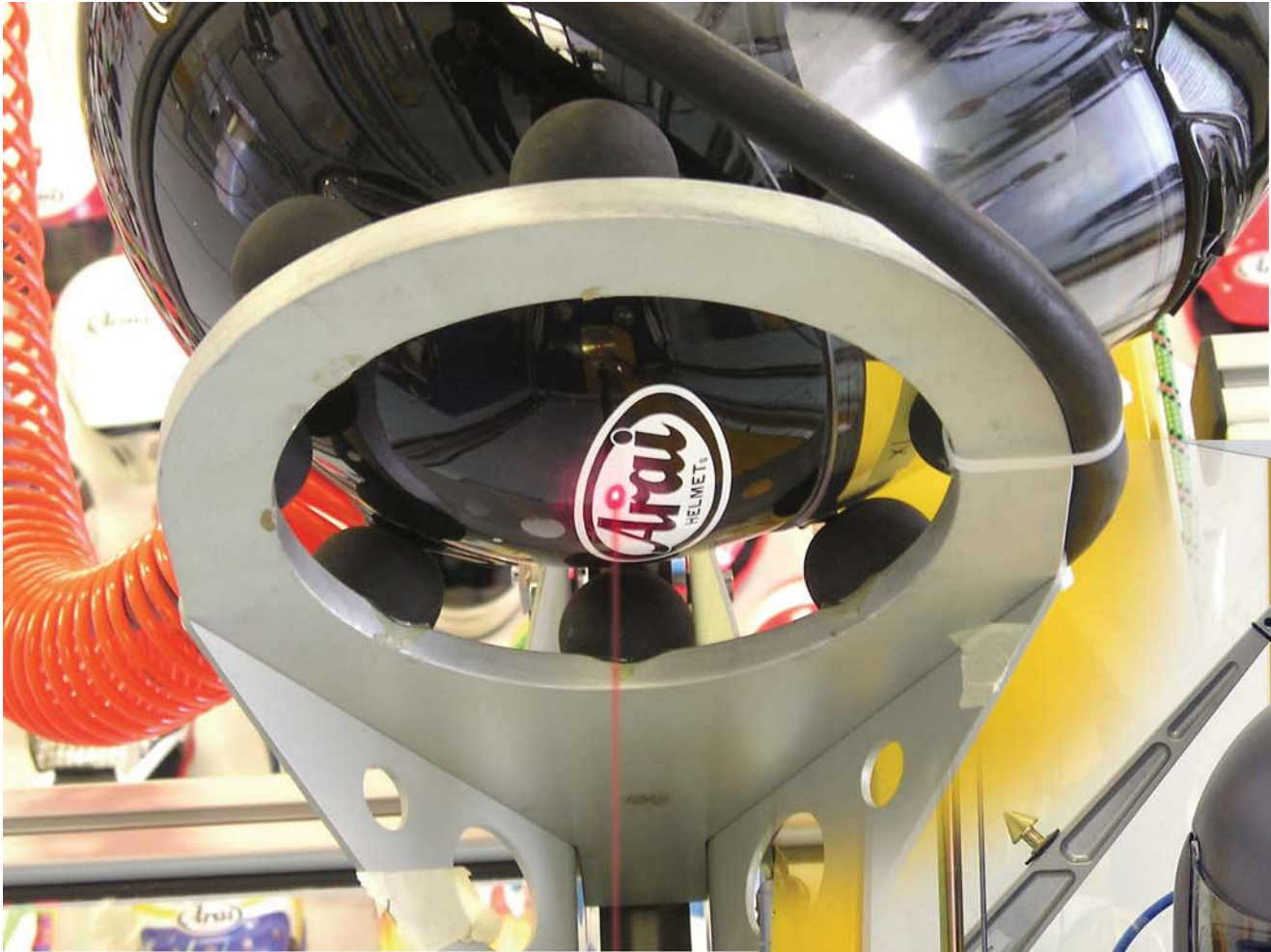
Laser beam positioning of impact point
