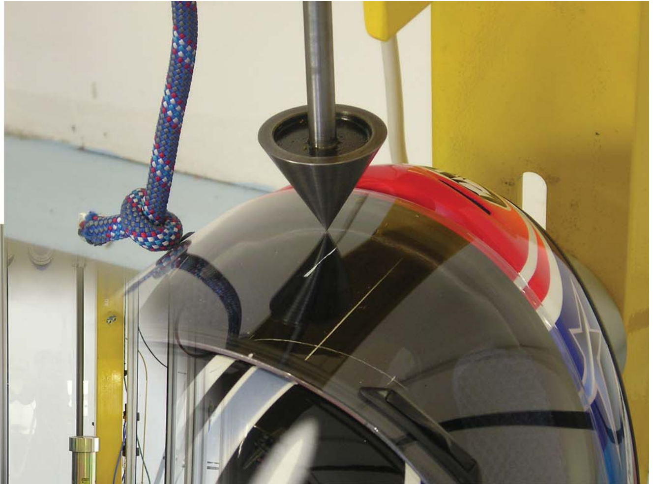
Visor penetration test
