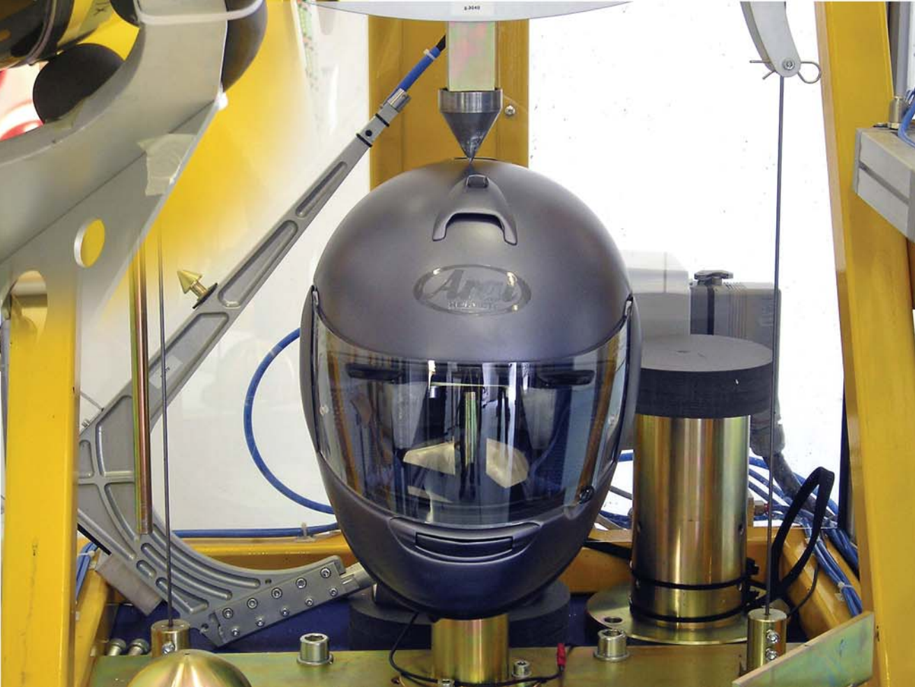
Positioning of penetration impact test striker (cone)
